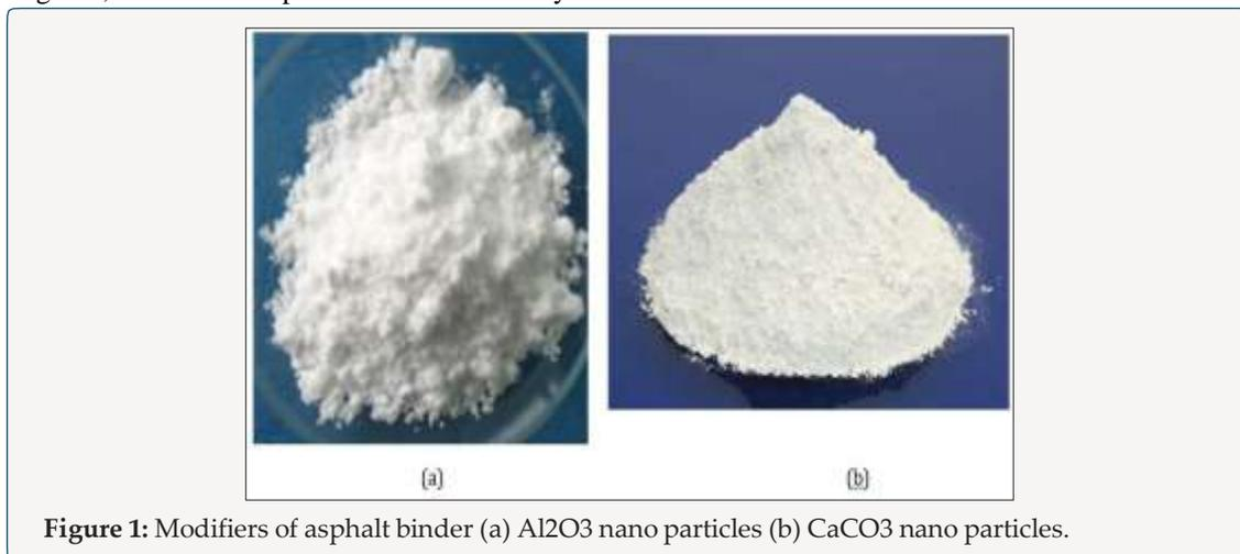
Figure 1: Modifiers of asphalt binder (a)  $Al_2O_3$  nano particles (b)  $CaCO_3$  nano particles.
