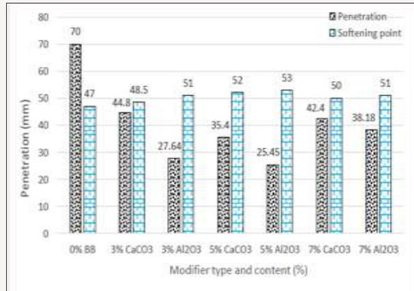
Figure 2: Penetration and softening point of modified asphalt binders.
